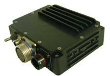
The 40A voltage regulator and powerbox is designed to be used in combination with a permanent magnet alternator. The variable three-phase input voltage from the alternator is full-wave rectified and smoothed to provide a DC low-impedance source to the regulator. The output voltage can be set to the customer's requirements.
